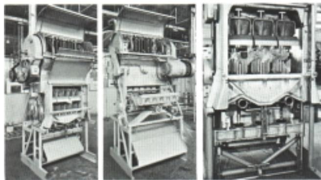
291 FRONT VIEW. The first model with positive rotary feeder. 291 BACK VIEW. The rotary feeder permitted the operating speed to increase to 75 strokes/375 fruit per minute. 491, FIRST MODEL TO USE 5" OIL RECOVERY CUPS AND ROTARY FEED. 60 strokes/180 fruit per minute.
