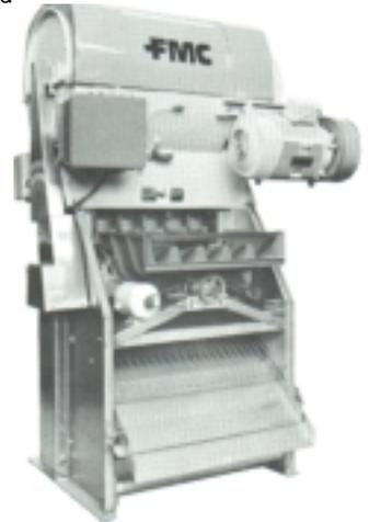
LATEST MODEL 291B. In-place clean-up & recycle peel oil recovery systems. 100 strokes/500 fruit per minute.
