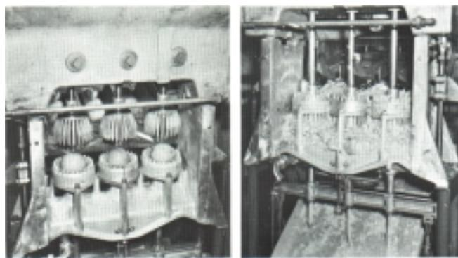
659 PROTOTYPE. Note the orifice discharge tubes at bottom which removed core, membrane and seeds from juice at the moment of extraction.
