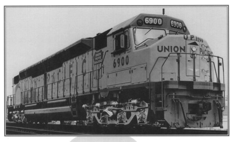
single unit diesel single unit diesel locomotives required four axle trucks to distribute their heavy weight and keep within track loading limits.
