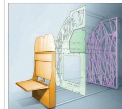
and to be strong enough to support the two fold-down seats on which flight attendants sit. It must be able to withstand impacts of up to 16 G. Oh, and it also must be less than 1-inch thick and attach to the plane in only four places to keep down the weight of connecting hardware.
