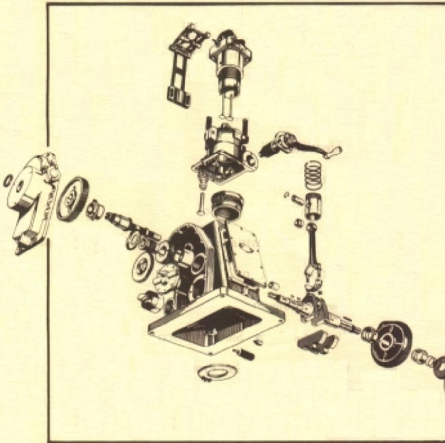
Exploded view of an early model CFR engine.
