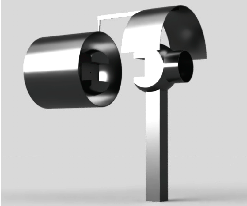
CAD drawing of the autographic recording mechanism of the Thurston Torsional Testing Machine, circa 1880. The pendulum arm and rectangular specimen grip is shown as the vertical element. The torsional load vs angular twist is recorded on the left hand cylinder. [CAD drawing by Priscilla Chang, BSME'21]
