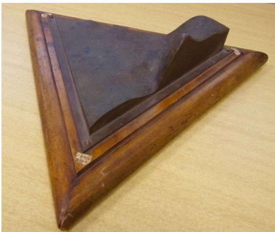
3 D plot in brass of the torsional strength of copper alloy as a function of percent alloy composition; Copper, Tin, Lead. Data taken from the Thurston testing machine, circa 1885
