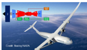
Parallel Gas-Electric Hybrid
