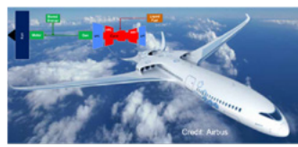
Full Series Turboelectric Hybrid
