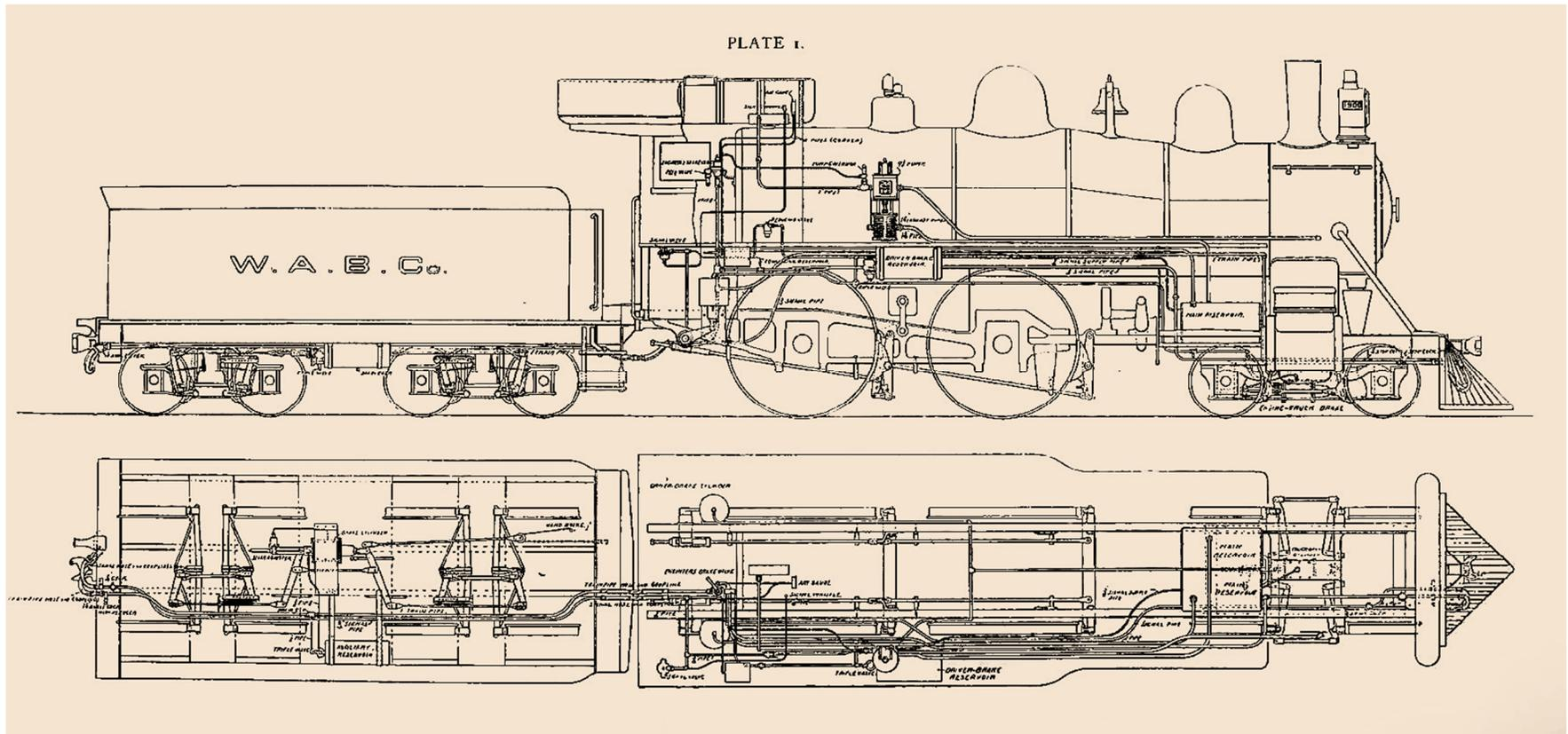
Above: Locomotive and Tender, equipped with a Westinghouse Automatic Air Brake System. The steam-air pump is shown located on the side of the locomotive, above the main drive wheels. A valve in the locomotive cab gave the operator control of the system, which applied brakes to all railcars on the train. From Air Brake Instruction Book of the Westinghouse Air Brake Company, 1901.
