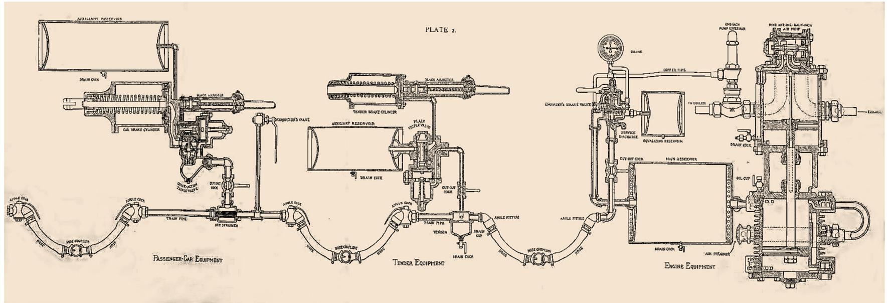
Above: Illustration of Westinghouse Automatic Air Brake System. The steam-air pump is shown at right, along with the control equipment located in the locomotive. At middle is the typical equipment installed in the tender, and at left the braking equipment installed in each passenger car. From *Air Brake Instruction Book of the Westinghouse Air Brake Company*, 1901.
