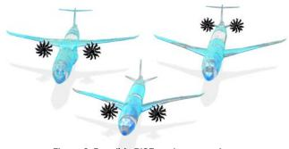
Figure 2. Possible RISE engine mounting positions on single-aisle airframes.
