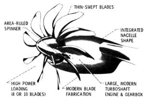
Figure 3. NASA 1980 high speed turboprop propulsion system. <sup>[4]</sup>
