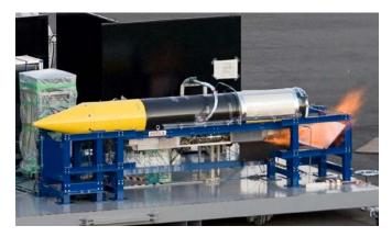
Figure 2. Sea Level Static Experiment of PCTJ.
