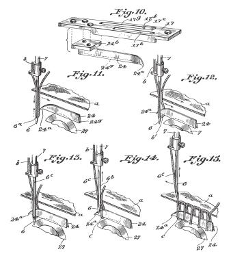
FIG. 2: A DRAWING INCLUDED IN MOENCH'S PATENT APPLICATION DONE BY MOENCH HIMSELF. HERE, MOENCH IS SHOWING HOW THE NEEDLE MAKES LOOPS AND IS CUT BY A BLADE.
