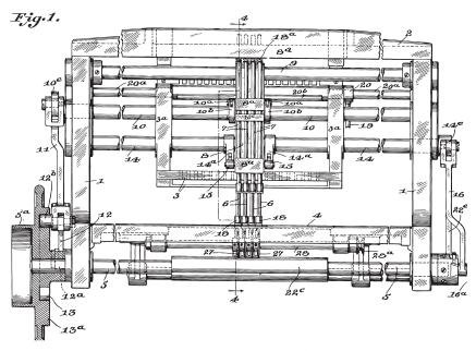
FIG. 3: ANOTHER DRAWING INCLUDED IN MOENCH'S PATENT WHICH SHOWS THE MACHINE IN FRONT ELEVATION.
